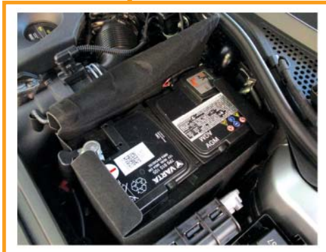
12 V Battery in Engine Compartment
