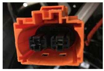
The electrical connectors are a new component developed for advanced accidental contact protection.
