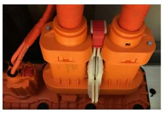
All HV wires in the ID.4 are connected mechanically.
