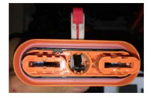
Shielding of the high-voltage wires is not required. The EMC measures are implemented in the high-voltage components by the EMC filter.
