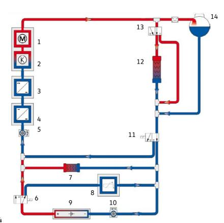
The J840 Battery Regulation Control Module controls thermal management of the high-voltage battery. In the version with a heat pump, it regulates the V683 Mixing Valve for High-Voltage Battery Warming, V696 Mixing Valve 2 for High-Voltage Battery Warming and the V590 High-Voltage Battery Coolant Pump.
