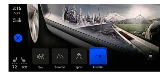
The vehicle does not switch into ECO mode when the high-voltage battery is discharged. Instead, a yellow turtle is displayed in the dash panel insert and the power output is reduced.
