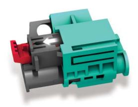
The fuse SC28 has a small "flag" on it. When removed, terminal 30 A is disconnected. The small "flag" is attached to allow quick removal without tools. The small "flag" can be replaced separately and the fuse is commercially available.
