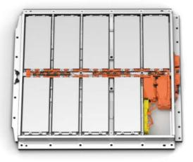
12 battery modules 82 kWh gross 77 kWh net
