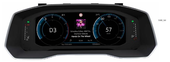
In the Digital Cockpit the analog gauges are presented virtually. The following warning lights, relevant to driver safety, are still set indicators and are available separately on the screen:
