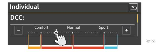
A slider (virtual slide control) for DCC is used for the first time in the Arteon. This makes the following possible:
