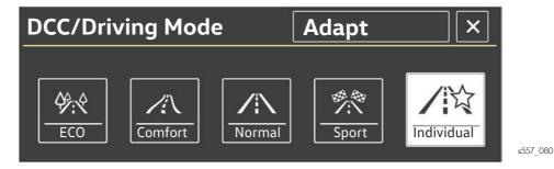
The "Individual" menu option allows the driver to customise the characteristic curves with infinitely variable adjustments.
