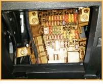
The N253 is located in the main fuse box. The electrical supply to the engine compartment, with the exception of the ABS Control Module J104 and Power Steering Control Module J500, is cut off by the N253 and when an airbag is deployed. This allows continued steering and braking.
