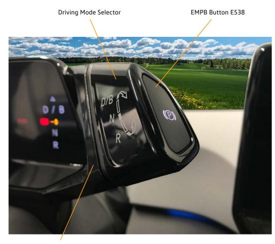
Steering Column Switch Module with J527
