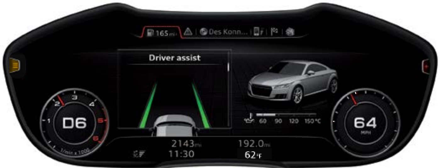
Representation of the system status of Audi active lane assist (not available for MY16)
