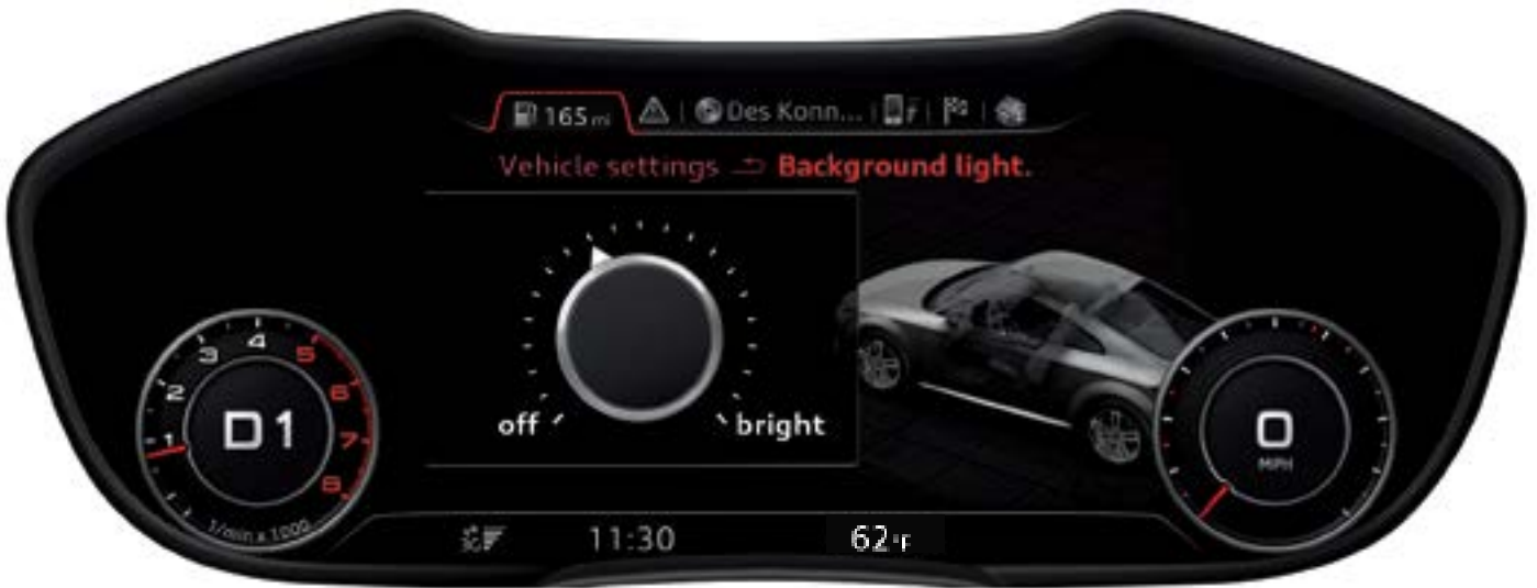
Settings menu for ambient lighting level
