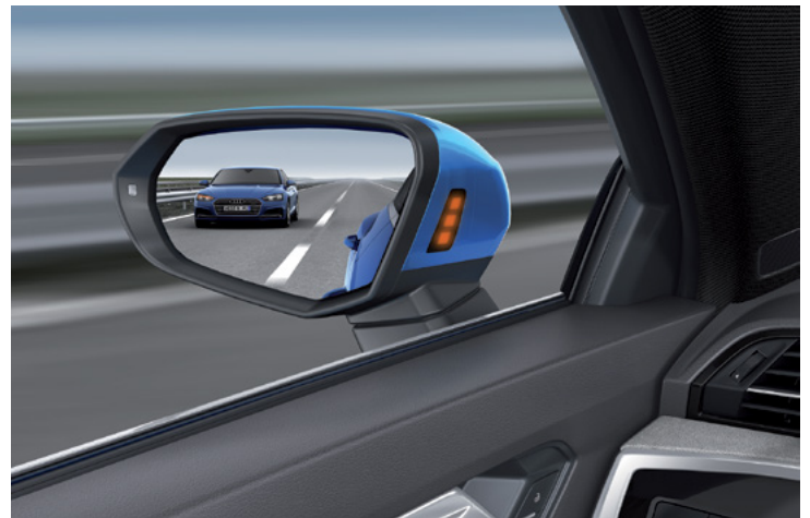
Active warning Audi side assist in left exterior mirror
