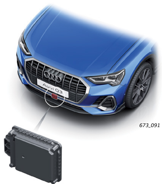
Lane Change Assistance Control Module J428 and Right Adaptive Cruise Control Sensor G259
